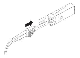
Figure 32. Inserting an LC-LC Fibre Channel cable into an SFP module
